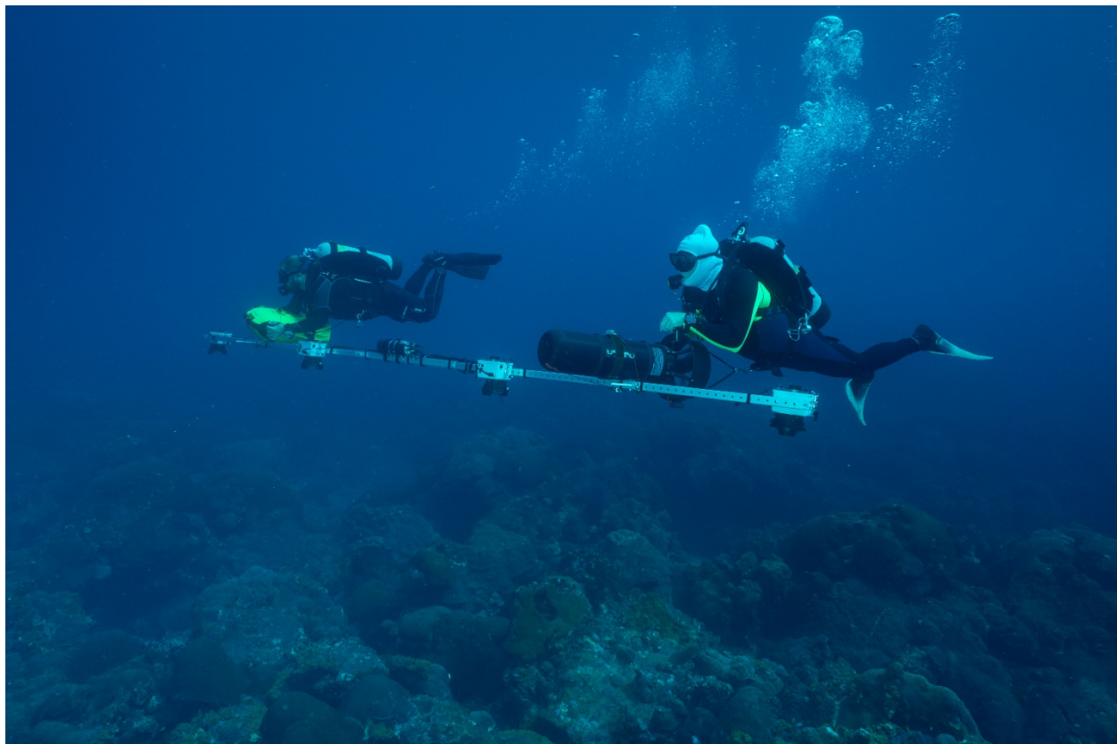
Divers use scooters to collect the imagery needed to build the mosaics. Photo: G.P. Schmahl/NOAA
