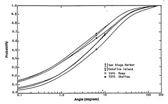
Fig. 1. Single scattering distribution functions for various water types (from Petzold<sup>3</sup>).
