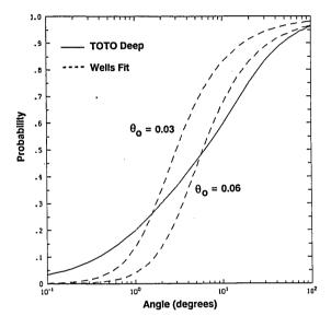
Fig. 2. Comparison of TOTO measurements of the scattering phase function with Wells's algebraic fit. For deep TOTO waters, Wells's model agrees with the median scattering angle if  $\theta_0 = 0.06$  rad. Data are from Petzold.<sup>3</sup>
