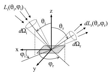
Fig. 1. Geometry used in the definition of the BRDF. The reflecting surface lies in the x-y plane; the z axis is normal to the surface.
