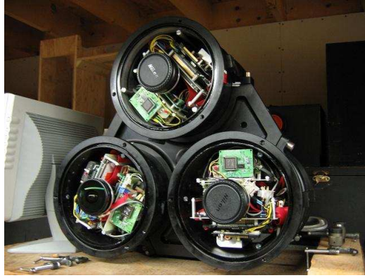
Fig. 1. Polrads assembly with three NuRADS cameras in a triangular arrangement. Shown without the cover plates, and glass dome windows.
