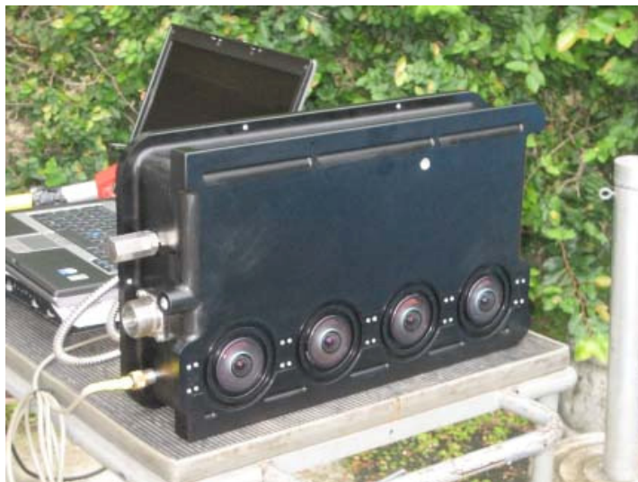
Fig. 2. Picture of the top of the polarization camera system. One can see the 4 fisheye lenses all aligned in a row. On the left are connectors to allow the system to be used, either over a dedicated cable (the big connector) or through the ROV system.
